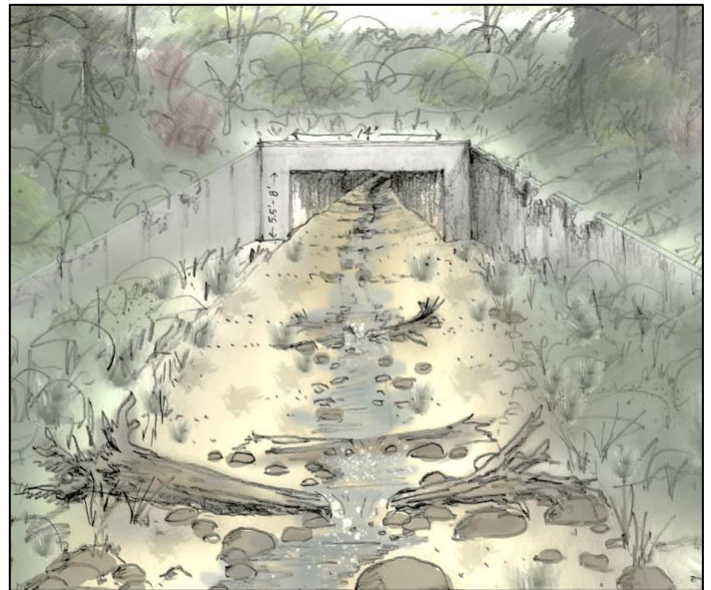
Conceptual drawing of finished culvert with creek flowing under 45th Ave. SW. Courtesy of Seattle Public Utilities
