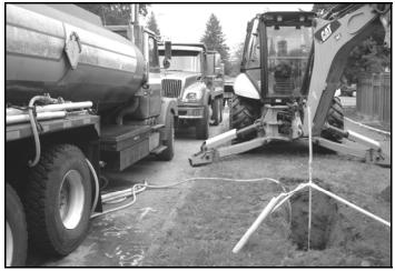
Pits like this one tested how quickly water soaked into the soil at shallow depths. Photo courtesy King County
